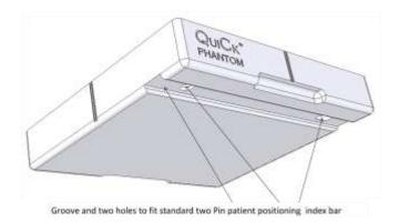
The top and four sides of the phantom are engraved to facilitate accurate setup in all orientations.
