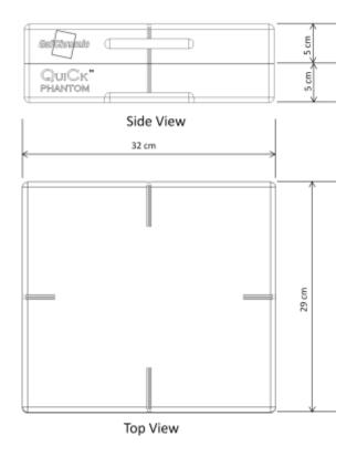
Phantom Body: Two slabs of CIRS Plastic Water<sup>™</sup> water-equivalent to within 1% from 150 keV to 25 MeV
