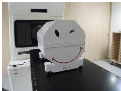
Fig 2 The Octavius phantom, with insert for positioning 8"x10" EBT3 film
