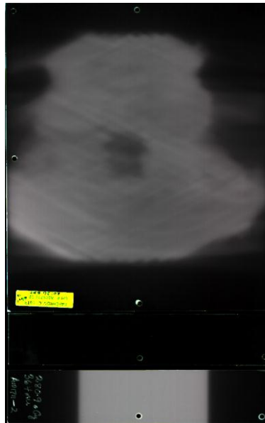
Figure 2: Dose Image: Application film with exposed and unexposed calibration films
